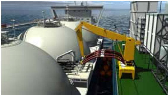
The loading system during coupling of the flexible pipes
