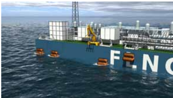
The loading and fender system waiting for approach of a shuttle tanker
